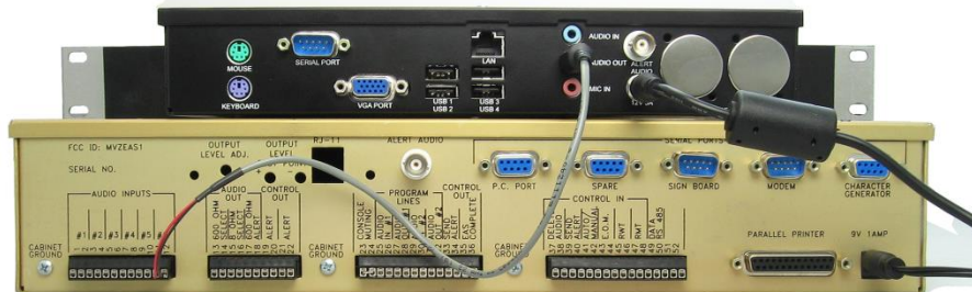
Connected Gorman-Redlich CAP-DEC 1 and EAS1 units (universal intermediary device configuration)
