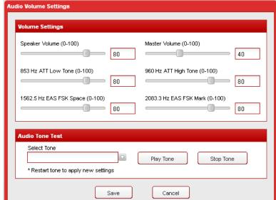
**853 Hz ATT Low Tone** – Sets the volume (0-100) for the 853 Hz tone that's used to generate the Attention tone (The default is 40). This setting should be set to half the desired Attention tone volume and should be the same volume as the 960 Hz tone.
