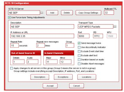
**Use Force-tune Timing Adjustments** – Select this option to use the force-tune time adjustments (from the Playback Options screen) for SCTE-18 messages.
