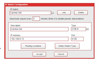
outputs on all configured IP switches. Enter zero (0) to disable periodic deactivations.
