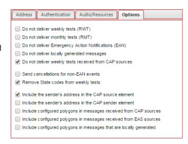
Do not deliver locally generated messages – If enabled, prevents messages that are generated locally (by an operator or automatic RWT generator) from being delivered to the selected server.
