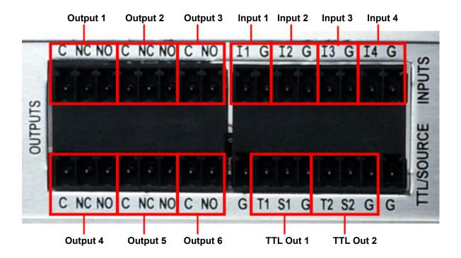
**General Purpose Outputs** – Six (6) contact closure outputs (switches) are provided for activating equipment to route the alert audio and video, sound alarms, and activate other devices during EAS transmission. When an output is active, the common and normally opened terminals are shorted together (closed).
