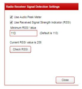
**Minimum RSSI Value** – When configured to use RSSI, this sets the minimum RSSI value for determining if the signal is present. If the measured RSSI is lower than this value, the signal will be considered bad.
