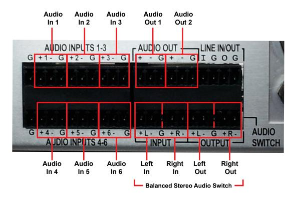
**Audio inputs** – Six (6) balanced 600 ohm audio inputs are provided to monitor external audio sources for EAS. They can be connected to audio sources such as external radio receivers, TV tuners, and satellite receivers. Configuration is provided to select between external audio sources and internal radio receivers for each input.
