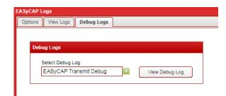
**EASyCAP Transmit Debug** - Includes debug information from processes that deliver alert messages to downstream servers and devices, such as SCTE-18 and DNCS recipients.
