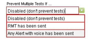
For a weekly test, the **Prevent Multiple Tests** option can be configured to prevent multiple RWT's from being transmitted during the week, where a week is considered to be Sunday at midnight until Saturday at 11:59:59.
