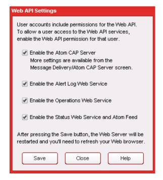
**Enable the Operations Web Service** – When enabled, a Web Service is available to allow https clients to perform operations like aborting a message in progress or confirming a pending message. Requires a Network Management license.
