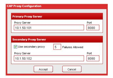
enabled, if a configurable number of sequential failures occur while polling a CAP source, the software will failover (or fall back) to the alternate proxy. Note that any unexpected response from a CAP source will be considered a failure.
