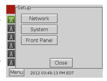
**Close button** – Exits the **Setup** menu and returns to the **Main** screen.
