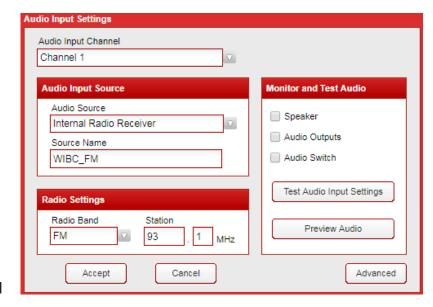
**Source Name** – Enter a descriptive name to identify the audio input. This name will be displayed on the Front Panel LCD and in the Logs to identify the audio input channel.
