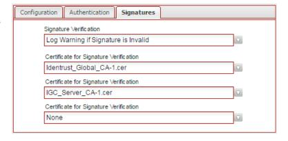
• Certificate for Signature Verification – Select the certificates required for the EASyCAP to verify the digital signatures of the CAP messages received from the selected IPAWS Atom feed. Up to three certificates may be necessary to complete the certificate chain. The EASyCAP will not attempt to download intermediary certificates.
