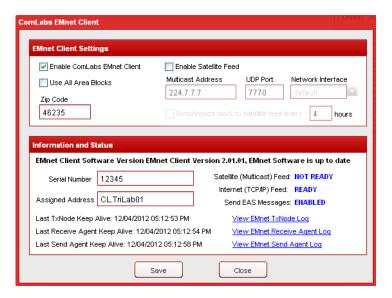
Multicast Address – Enter the multicast address of the satellite receiver.
