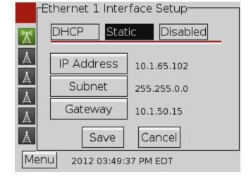
**Subnet button** – Displays a menu with a keyboard to enter the interfaces subnet mask.
