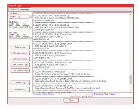
The system log will be displayed as shown above. One hundred log records are displayed at a time. Use the << (First), < (Previous), > (Next), and >> (Last) buttons to navigate through all of the log records.
