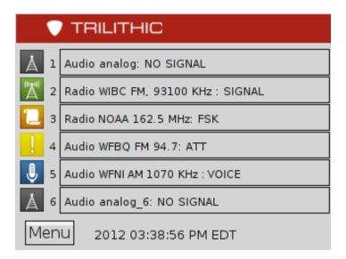
The Main screen is displayed when the system is idle and monitoring for EAS messages. The EASyCAP® application type and software version are displayed in the top right corner of the screen. The bottom line shows the current date and time of the EASyCAP®.
