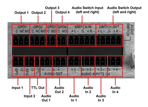
**General Purpose Outputs** – Four (4) contact closure outputs (switches) are provided for activating equipment to route the alert audio and video, sound alarms, and activate other devices during EAS transmission. When an output is active, the common and normally opened terminals are shorted together (closed).
