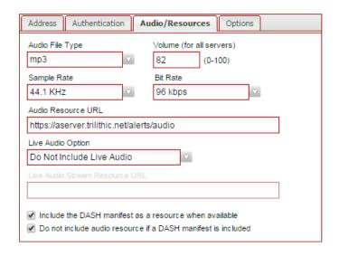
**Audio Resource URL** – This setting is used to construct the CAP message audio resource URI. The CAP message audio resource URI is constructed by appending the audio filename to the text that is configured here.
