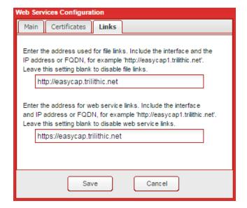
Press the **Save** button to save configuration changes and install or generate a new Web Server certificate if configured. Press the **Cancel** button to exit without saving changes.
